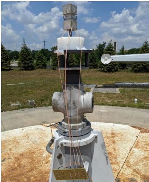
Fig. 8. QSCA single element prototype with quadrature feed board, tested at AAMI.
