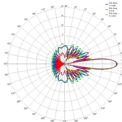
Fig. 4. Slot array principal azimuth cut overlays.
