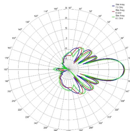
Fig. 4. Slot array principal elevation cut overlays.
