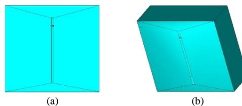
Fig. 1. Slot antenna model: (a) front view; (b) isometric view.
