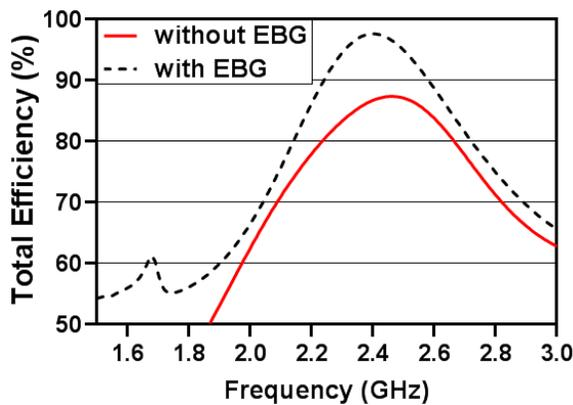
Fig. 3. Antenna efficiency with and without EBG.
