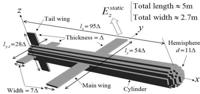
Fig. 3. A realistic aircraft model discretized by 9449 cubic PEC cells. The tail wing is placed at the center of the cylinder, while the main wing position is one  $\Delta$  beyond the tail wing towards the  $z$  direction. The cylinder lies along the  $x$  axis and the main wing along the  $y$  axis.
