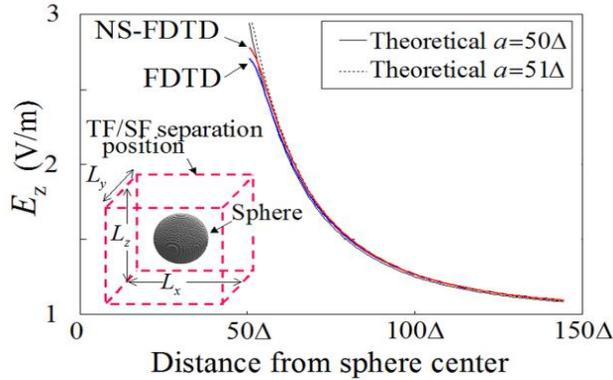
Fig. 2. Variation of the ESF ( $E_z$ ) component vs. distance (along the  $z$ -axis) from the sphere center, derived by various methods. The applied field, with  $E_0 = 1$  V/m, is parallel to  $z$  axis. The theoretical values via (3) are shown for the cases of  $a$  and  $a + \Delta$ , since a discretized cell model has an ambiguity of one  $\Delta$  in the FDTD algorithm. The TF/SF separation area size is  $L_{x,y,z} = 290\Delta$ .
