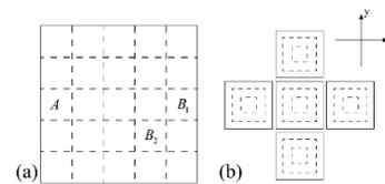
Fig. 1. (a) A two-dimensional power relay plane.  $A$  is the start unit, and  $B_1$ ,  $B_2$  are two locations of the receiver. (b) Each unit can transfer power to its adjacent units in  $x$  and  $y$  directions.
