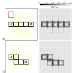
Fig. 3. (a) A  $5 \times 5$  matrix model. Power transfer route from A to  $B_1$  is high-lighted on the left. In the red box is the model of single unit. On the right is the power flow. (b) Power transfer route from A to  $B_2$  on the left, and power flow on the right.
