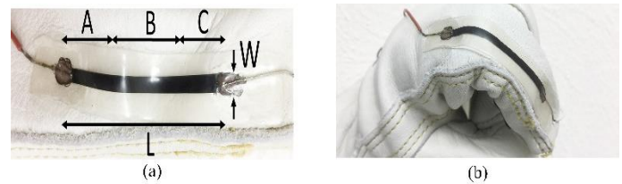
Fig. 1. (a) Highly stretchable strain sensor based on electrospun carbon nanofibers and distribution of the Strain Sensor (Dimensions (in mm): A = 1.31, B = 27.6, C = 0.99, W = 2.86 and L = 29.9). (b) Distribution of the strain sensor over the finger using a glove.
