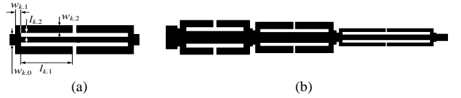
Fig. 2. CMRC-based three-section impedance matching transformer: (a) compact microstrip resonant cell (CMRC) cell; and (b) transformer geometry.
