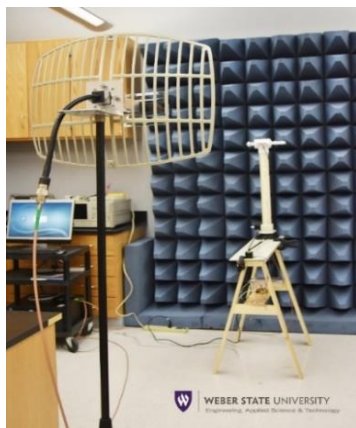
Fig. 1. Principal plane pattern measurement setup for the Yagi-Uda prototype.
