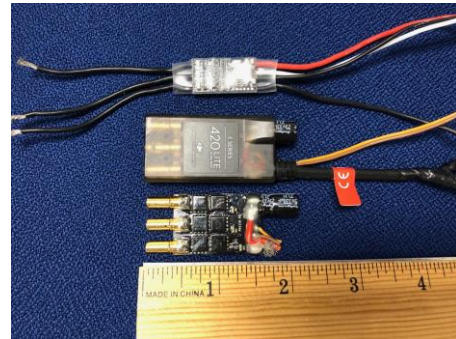
Fig. 1. Electronic speed controllers (ESC), BL Heli (top) and: DJI 430 Lite (middle and bottom).
