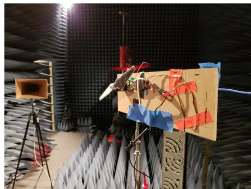
Fig. 2. DJI ESC experimental setup.
