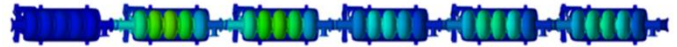
Fig. 2. The longitudinal cavity mechanical mode displacement profile at longitudinal plane in PIP-II 650 MHz SRF CM.
