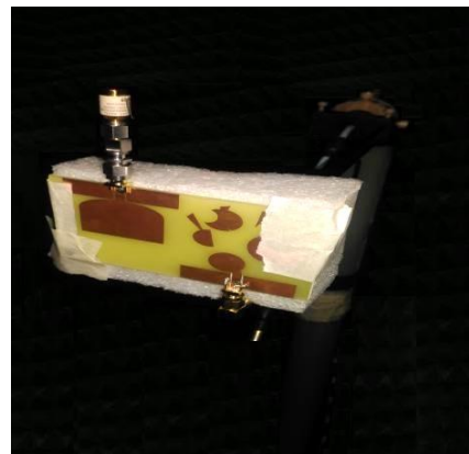
Fig. 13. Radiation pattern measurement setup at ARC, UiTM, Shah Alam, Malaysia.
