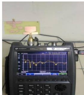
Fig. 4. Measurement setup of UWB antenna.
