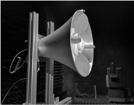
Fig. 17 The antenna under testing in a microwave anechoic chamber.
