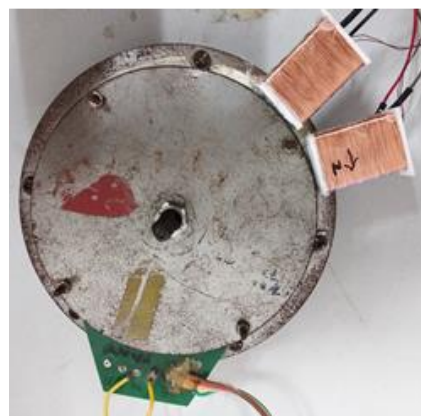
Fig. 14. Installation position of fluxgate detector.
