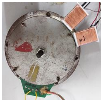
Fig. 14. Installation position of fluxgate detector.
