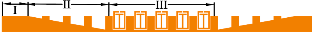
Fig. 3. The schematic of the proposed spoof SPP based bandstop filter with capacitively loaded RSS.
