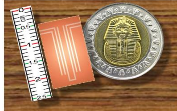
(b) S-band BPF for the downlink
