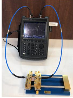
(b) Measurement of the transmission coefficient |S_{21}| using the VNA
