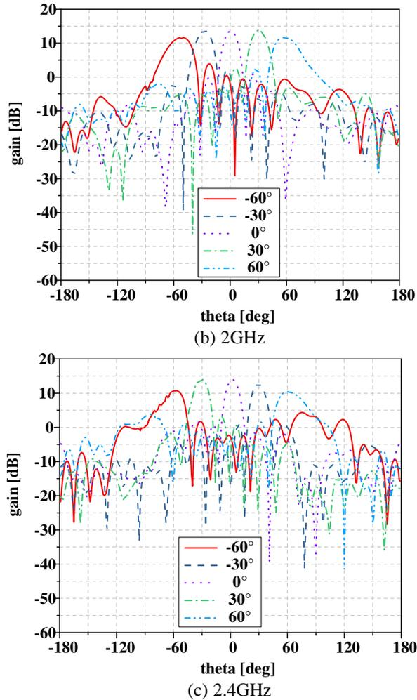
Fig. 10. Measured scanning performances of configuration array 1 for  $-45^\circ$  polarization at different frequency.
