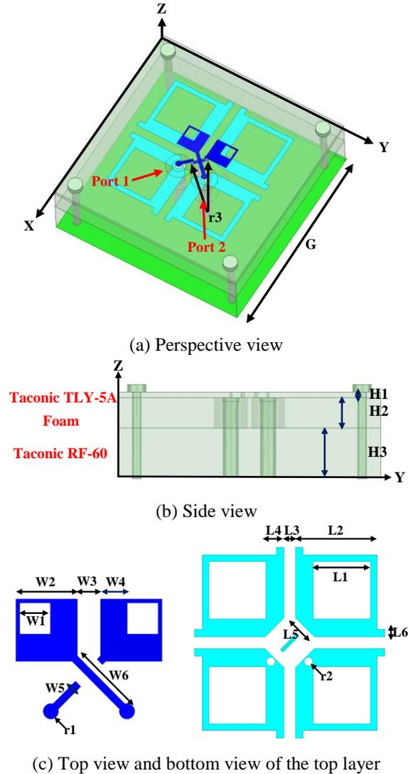
Fig. 1. Configuration of the dual polarized antenna.
