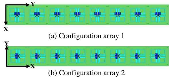
Fig. 6. Configuration of scanning linear array.
