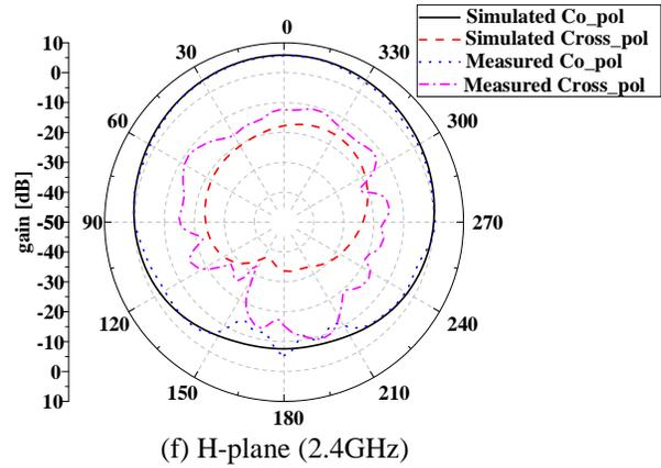
Fig. 5. Radiation patterns at 1.7GHz, 2 GHz and 2.4GHz for  $-45^\circ$  polarization.
