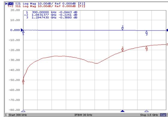
Fig. 5. S11 of coaxial fixture (partially shown in 300 KHz ~1.5 GHz).
