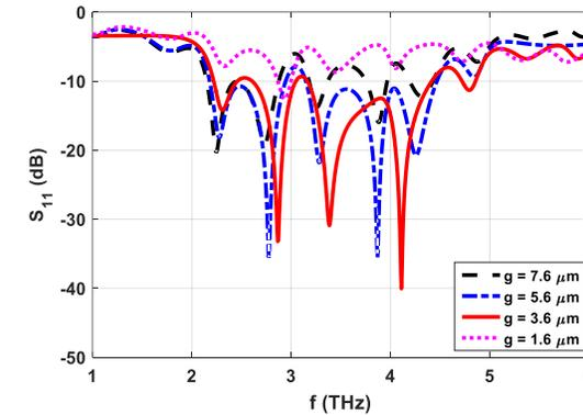
Fig. 10.  $S_{11}$  of THz antenna without lens with the variations in  $g$ .
