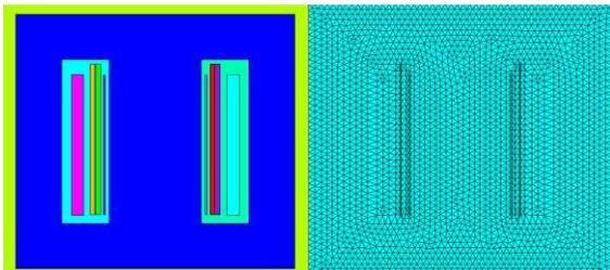
Fig. 9. The model and mesh of the transformer.
