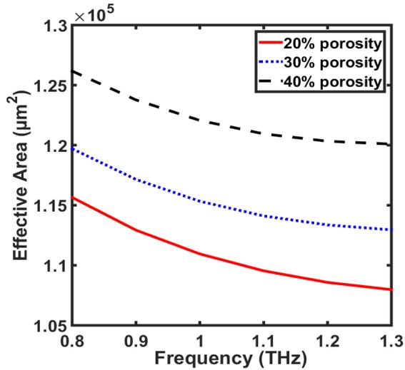
Fig. 7. Frequency-dependent effective mode area of the quasi TE mode at different porosity percentages.
