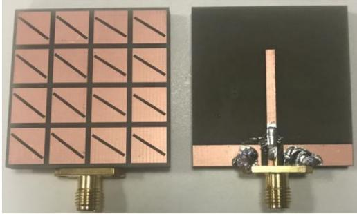
Fig. 7. Photographs of the fabricated antenna prototype.
