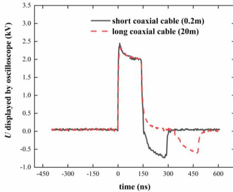
Fig. 13. The responsive waveforms of ZnO varistor with the 3 kV voltage and 150 ns pulse width inputted using the coaxial cable with different lengths.
