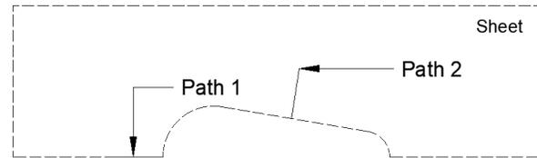
Fig. 10. Paths for monitoring the magnetic induction evolution.
