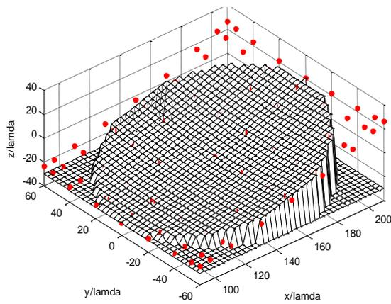
Fig. 11. Initial main reflector and control points.
