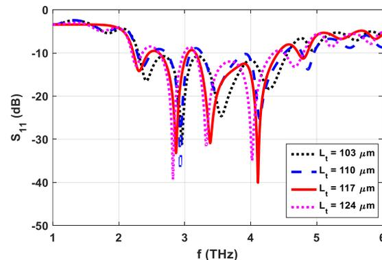
Fig. 6.  $S_{11}$  of THz antenna without lens with the variations in  $L_t$ .
