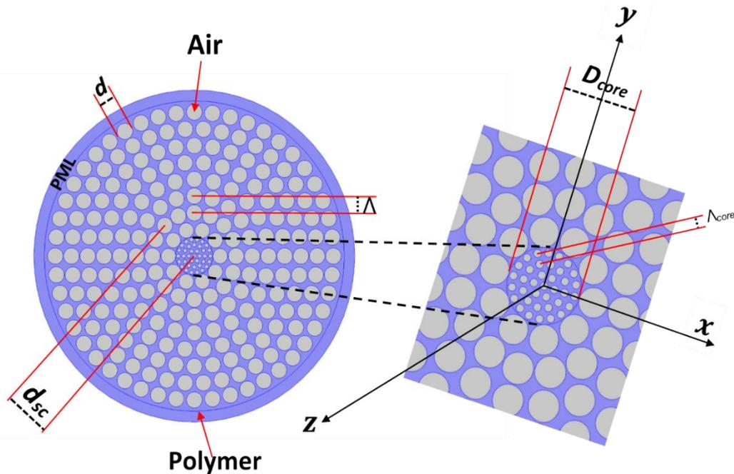
Fig. 1. Cross-section of the CCPCF with TOPAS as a background material.
