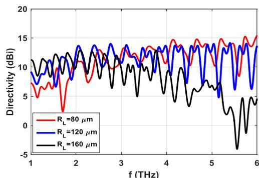
Fig. 12. Effect of variations in  $R_L$  on directivity of THz antenna with lens.
