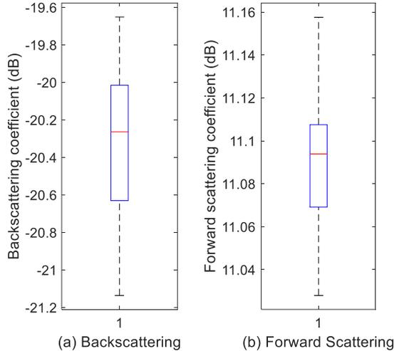
Fig. 5. Boxplot: backscattering and forward scattering coefficients by 2nd-order HOSPM among different frequencies.
