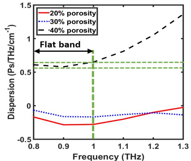
Fig. 11. The frequency dependent dispersion  $\beta_2$  at different porosity percentages.
