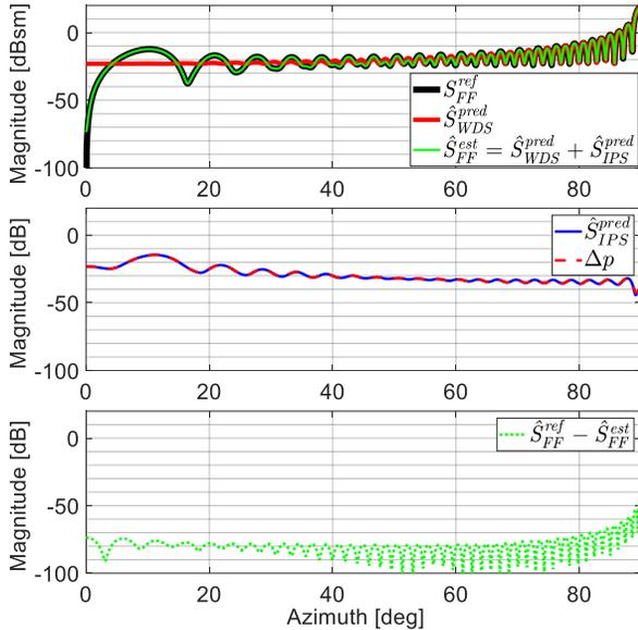
Fig. 4. Reference, WDP and IPS solutions for a flat plate (magnitude). Discrepancies between the reference and WDP solution (top) are corrected with an IPS solution (middle) to yield low reconstruction error (bottom).
