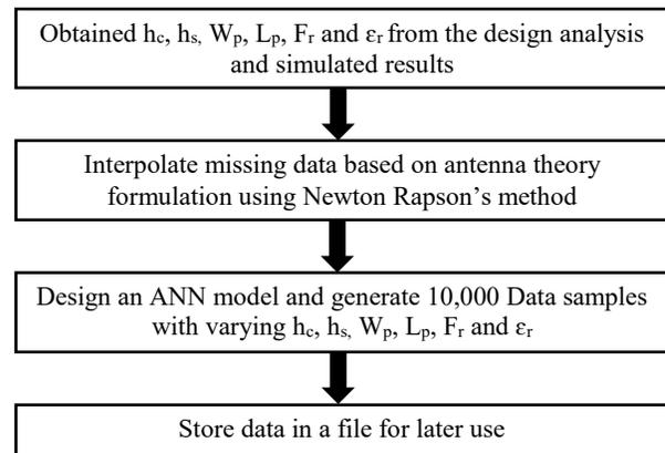
Fig. 2. Data acquisition and preparation block diagram.
