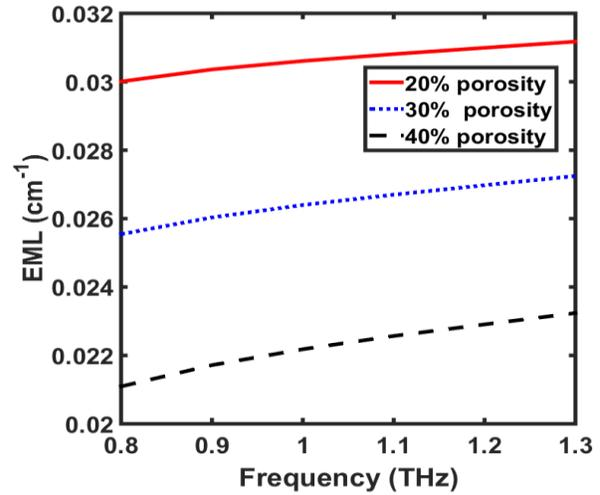
Fig. 5. EML versus the operating frequency at different porosity percentages.
