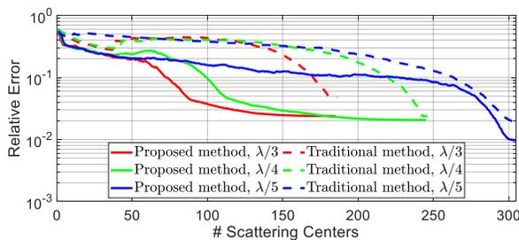
Fig. 11. Robustness of proposed and traditional method solutions for  $\lambda/3$  to  $\lambda/5$  discretizations of the angled plate.
