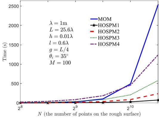
Fig. 3. Time cost by MOM and HOSPMs with 1st-, 2nd-, 3rd- and 4th-order (in the unit of second).
