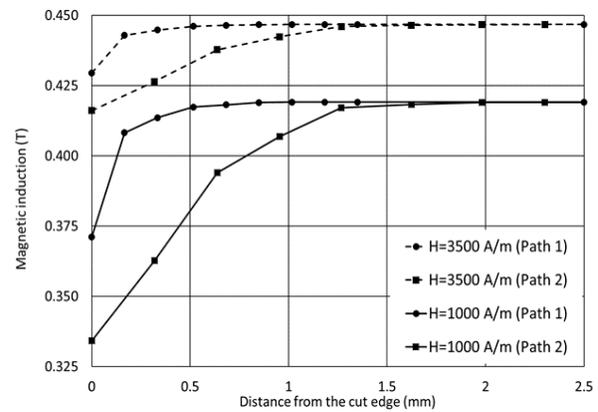
Fig. 11. Magnetic induction evolution along different paths.
