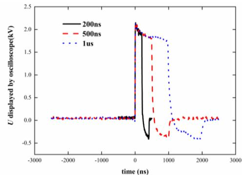
Fig. 12. The responsive waveforms of ZnO varistor with the 2.5 kV voltage but different pulse widths inputted.
