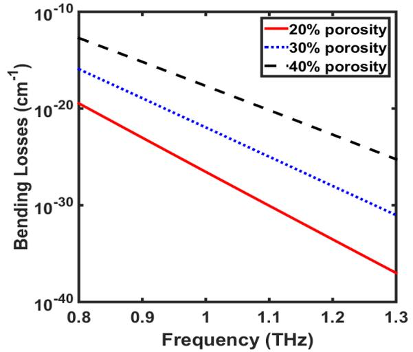
Fig. 8. Frequency-dependent bending loss of the quasi TE mode at different porosity percentages.
