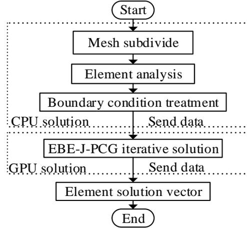
Fig. 1. Flow of CPU+GPU heterogeneous computing model of EBE-FEM.
