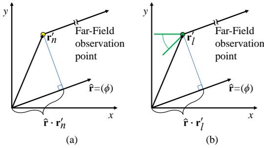
Fig. 1. Far-Field approximation of a (a) IPS and (b) WDP.
