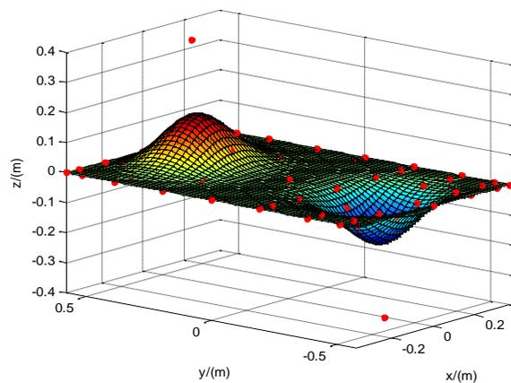
Fig. 7. Change value of two control points in Z coordinate to get the new surface.
