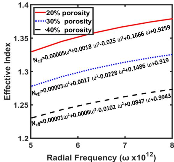
Fig. 10. The effective index  $N_{eff}$  of the quasi TE mode versus the radial frequency.
