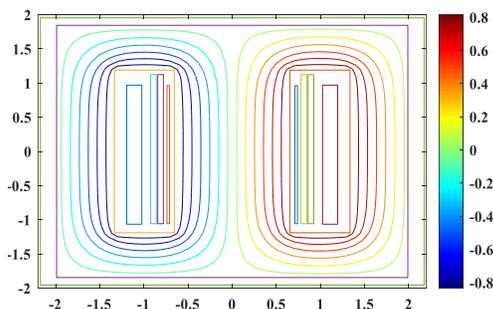
Fig. 10. Distribution of magnetic lines in transformer.
