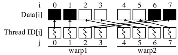
Fig. 4. Redirected thread-data mapping.
