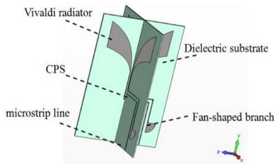
Fig. 1. The structure diagram of dual-polarized UWB antenna.
