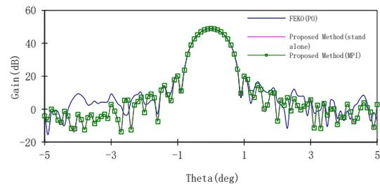
Fig. 9. Radiation pattern of the dual reflector antenna in different methods.
