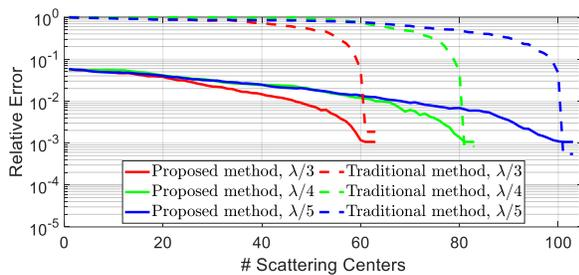
Fig. 10. Robustness of proposed and traditional method solutions for  $\lambda/3$  to  $\lambda/5$  discretizations of the flat plate.
