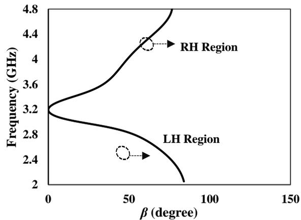
Fig. 7. Dispersion diagram of the proposed BLC.
