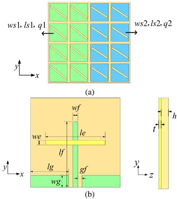
Fig. 3. Illustration of the geometry with the design parameters of the proposed antenna: (a) the top view; (b) the back view and the side view.
