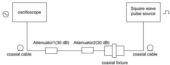
Fig. 3. Schematic diagram of experiment system.
