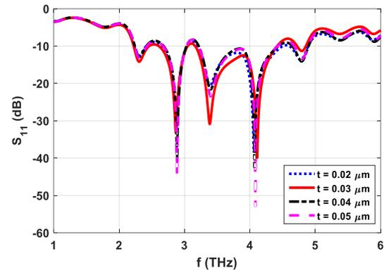
Fig. 4.  $S_{11}$  of THz antenna without lens with the variations in metal thickness ( $t$ ).
