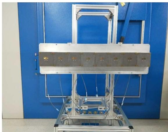
Fig. 9. Prototype of the scanning array.
