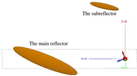
Fig. 10. Model of the dual offset Cassegrain antenna.
