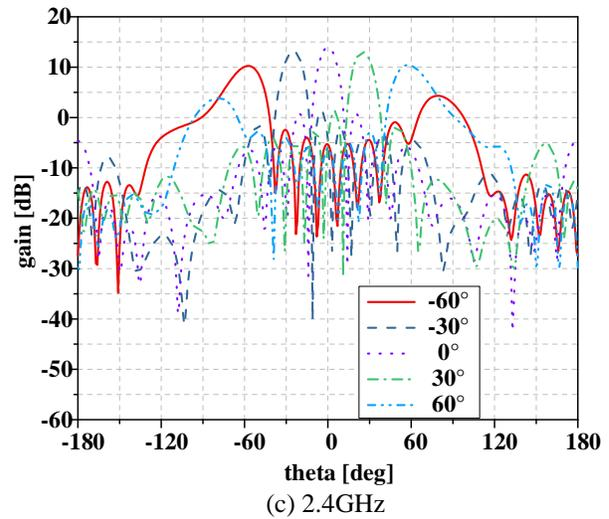
Fig. 7. Scanning performances of configuration array 1 for  $-45^\circ$  polarization at different frequency.
