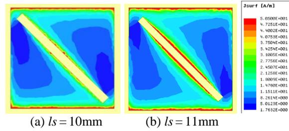
Fig. 2. Simulated surface current amplitudes of the PCMS at 5.75 GHz for different slot lengths.
