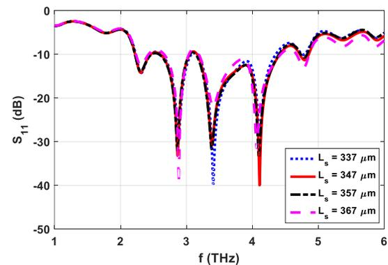
Fig. 5.  $S_{11}$  of THz antenna without lens with the variations in substrate length ( $L_s$ ).
