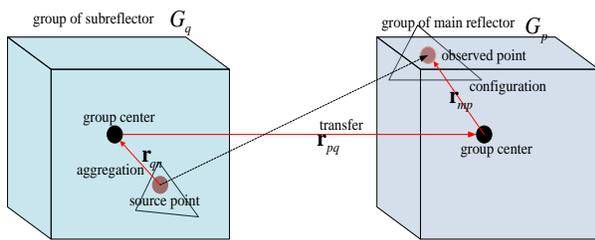
Fig. 3. Principle of accelerating the effect of the subreflector to the main reflector in single level.
