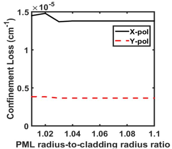
Fig. 2. Confinement loss of the quasi TE/TM mode versus the PML radius-to-cladding radius ratio.
