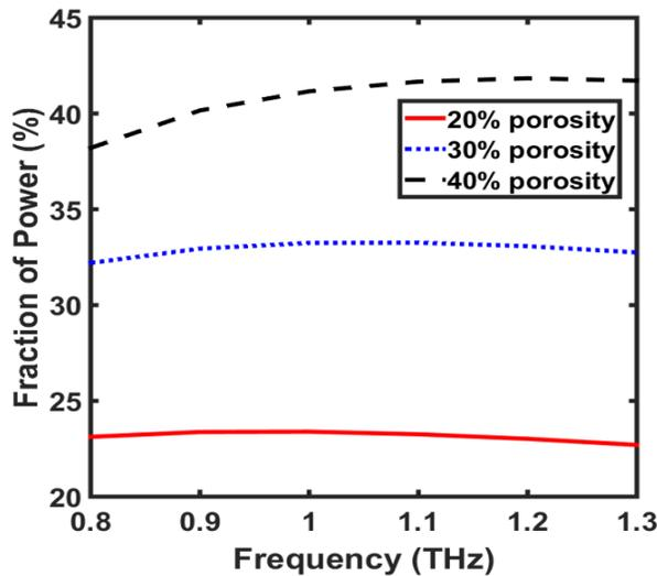
Fig. 9. The fraction of power percentage of the quasi TE mode through the core holes versus the frequency at different porosity percentages.
