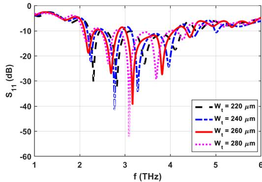
Fig. 8.  $S_{11}$  of THz antenna without lens with the variations in  $W_t$ .
