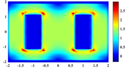
Fig. 11. Distribution of magnetic flux-density in transformer.
