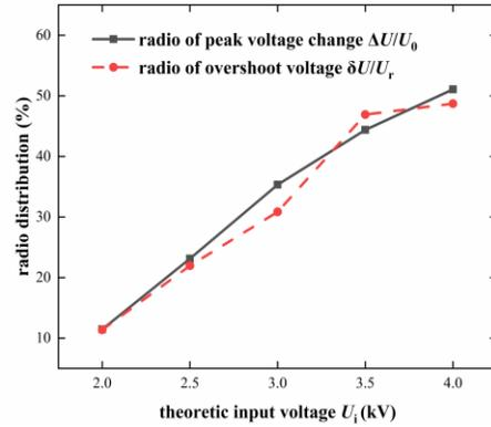
Fig. 10. The radio distribution of  $\Delta U$  and  $\delta U$ .
