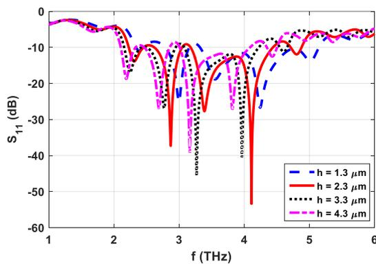
Fig. 3.  $S_{11}$  of THz antenna without lens with the variations in substrate thickness ( $h$ ).
