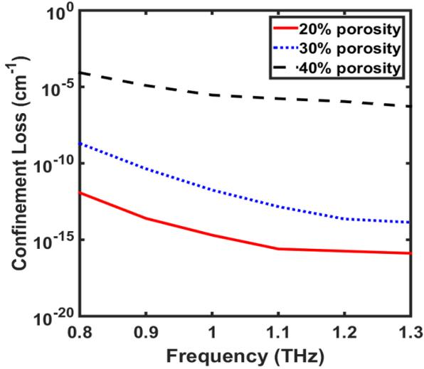
Fig. 6. Frequency-dependent confinement loss of the quasi TE mode at different porosity percentages.
