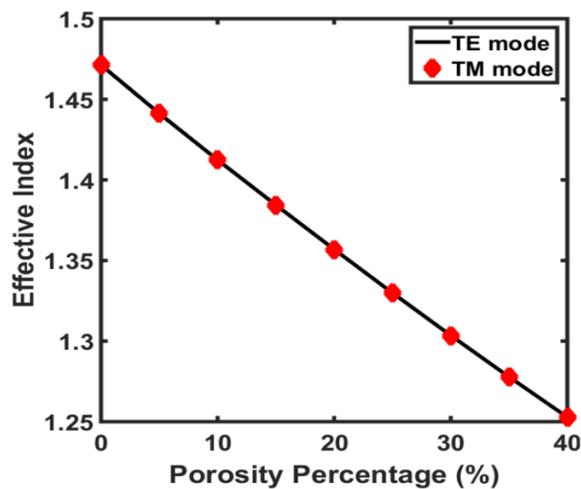
Fig. 4. The effective index of the fundamental quasi TE and quasi TM modes versus the porosity percentage (%).
