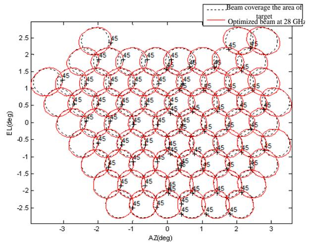
Fig. 13. Isoline pattern of the optimized beam at the frequency of 28GHz.
