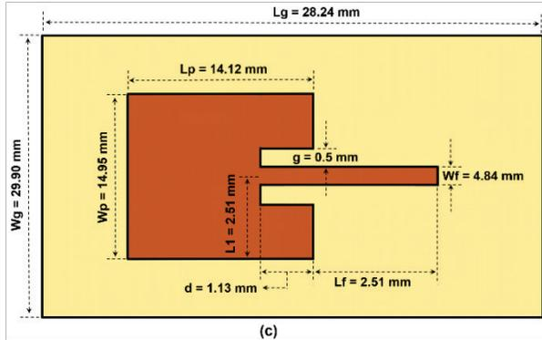
Fig. 1. Geometry of the proposed antennas with required dimensions at: (a) 28 GHz, (b) 24 GHz, and (c) 10 GHz.
