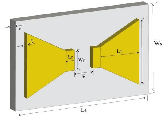
Fig. 1. Design of bowtie THz antenna.
