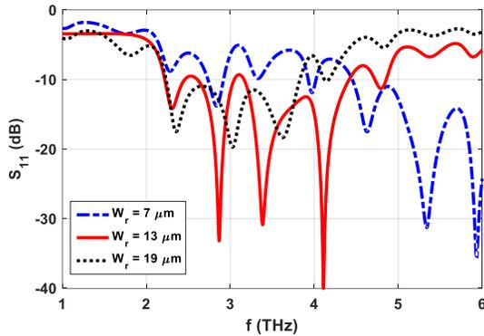
Fig. 7.  $S_{11}$  of THz antenna without lens with the variations in  $W_r$ .
