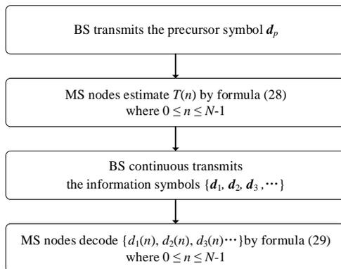
Fig. 4. Flow diagram of the RCED process.
