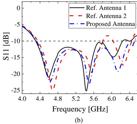
Fig. 6. (a) The AR, broadside gain and (b) the S11 of the proposed antenna and the two reference antennas with uniform PCMS array (the proposed antenna:  $(l_1, l_2, q_1, q_2) = (9.45\text{mm}, 8.80\text{mm}, 52.5^\circ, 57^\circ)$ ; Ref. Antenna 1:  $(l_1, q_1) = (9.45\text{mm}, 52.5^\circ)$ ; Ref. Antenna 2:  $(l_2, q_2) = (8.80\text{mm}, 57^\circ)$ ).
