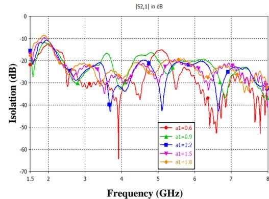
Fig. 5. Port isolation degree curves varying with  $a_1$ .
