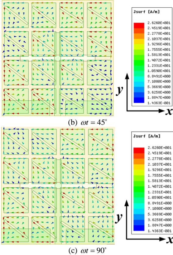
Fig. 5. Simulated surface current distributions of the proposed antenna at 5.3 GHz for different time instants.
