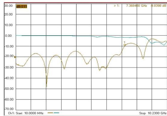
Fig. 6. S11 of coaxial fixture (partially shown in 10 MHz ~10.23 GHz).
