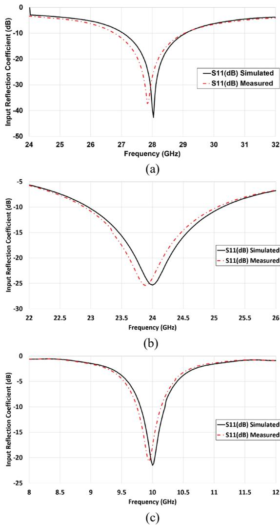
Fig. 5. Comparison of the measured and simulated results “input reflection coefficient” of a fabricated air substrate patch at: (a) 28 GHz, (b) 24 GHz, and (c) 10 GHz resonances.
