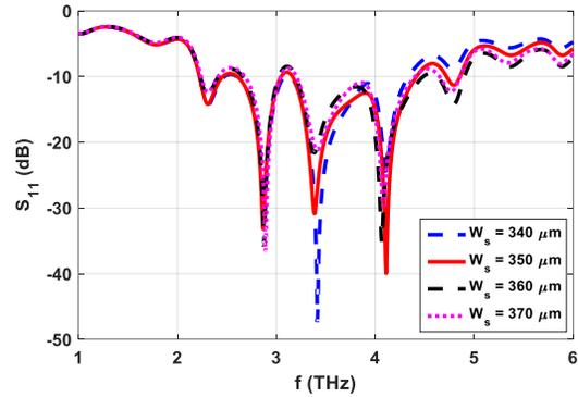
Fig. 9.  $S_{11}$  of THz antenna without lens with the variations in  $W_s$ .
