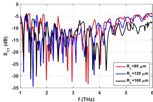
Fig. 11. Effect of variations in  $R_L$  on  $S_{11}$  of THz antenna with lens.
