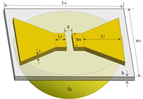
Fig. 2. Design of Bowtie THz antenna with lens.
