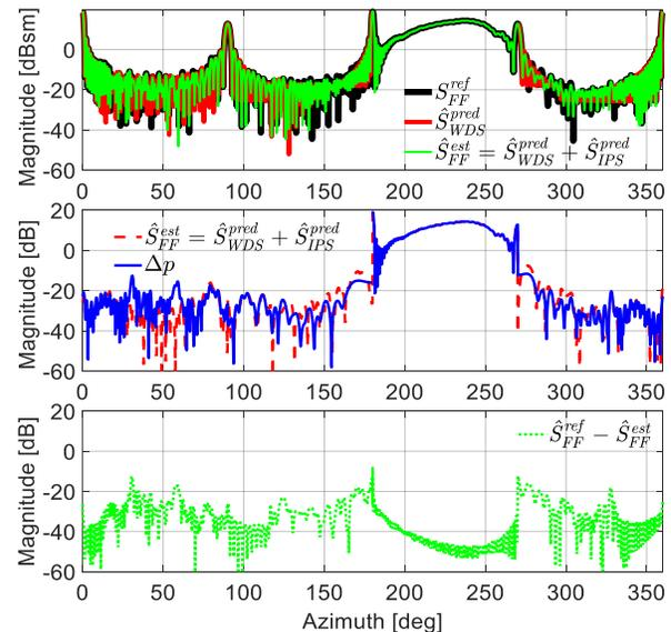
Fig. 8. Reference, WDP and IPS solutions for an angled plate (magnitude only). Discrepancies between the reference data and WDP solution (top) are corrected with an IPS solution (middle) to yield low reconstruction error (bottom).
