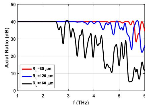
Fig. 13. Effect of variations in  $R_L$  on axial ratio of THz antenna with lens.
