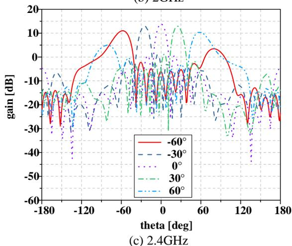
Fig. 8. Scanning performances of configuration array 2 for  $-45^\circ$  polarization at different frequency.
