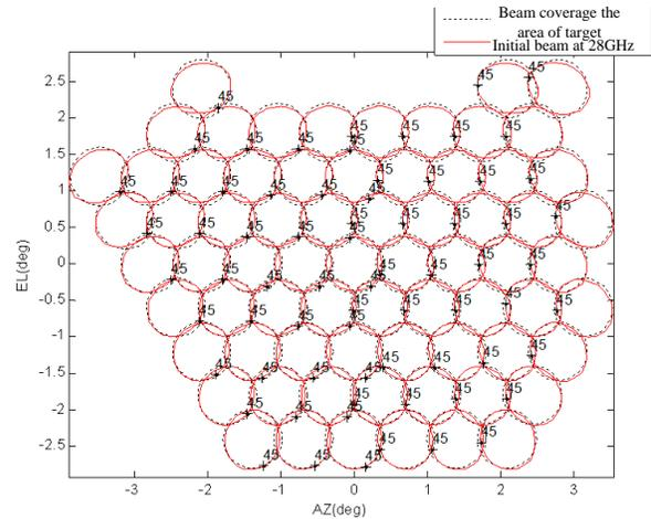
Fig. 12. Isoline pattern of the initial beam at the frequency of 28GHz.
