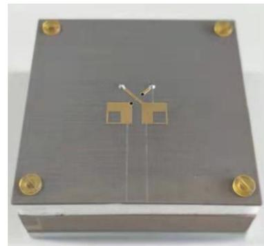
Fig. 2. Prototype of the proposed antenna.
