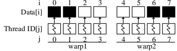
Fig. 3. Original thread-data mapping.
