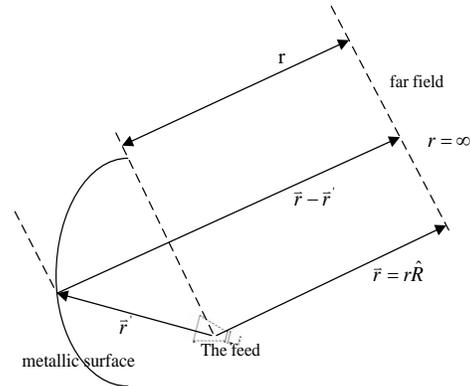
Fig. 1. Radiation of the single reflector antenna in PO.
