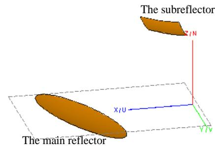
Fig. 8. Model of the dual offset Cassegrain antenna.
