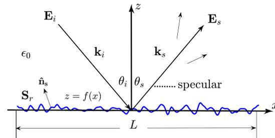
Fig. 1. Geometry for wave scattering by a conducting random rough surface.
