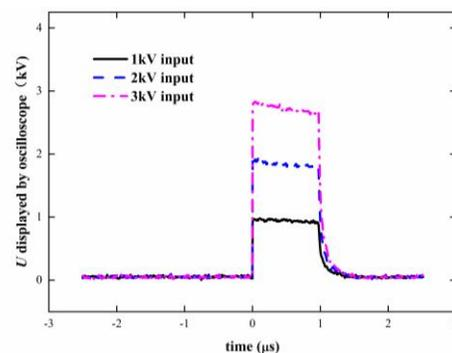
Fig. 7. Output waveforms of system without ZnO varistor fitted in.
