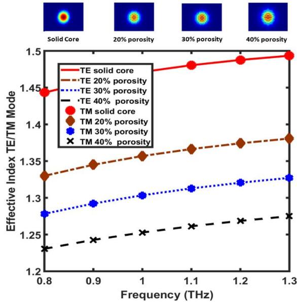
Fig. 3. The effective index of the fundamental quasi TE/TM mode versus the frequency at different porosity percentages. The inset shows the main electric field component of the quasi TM mode at different porosities.
