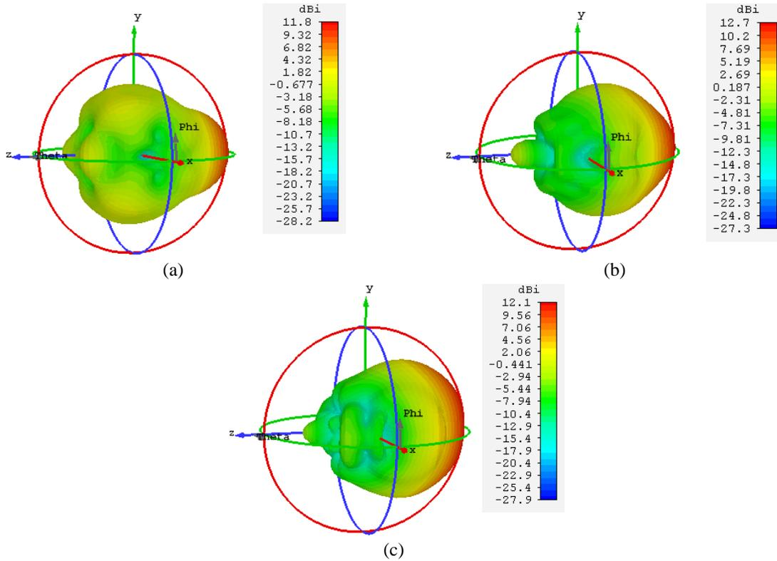
Fig. 18. 3D radiation patterns for different  $R_L$  values: (a)  $R_L = 80 \mu\text{m}$  at  $f = 2 \text{ THz}$ , (b)  $R_L = 120 \mu\text{m}$  at  $f = 2.1 \text{ THz}$ , and (c)  $R_L = 160 \mu\text{m}$  at  $f = 2.15 \text{ THz}$ .
