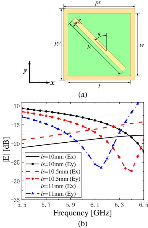
Fig. 1. (a) A unit cell of the PCMS, and (b) the amplitudes of the transmitted E-field components.
