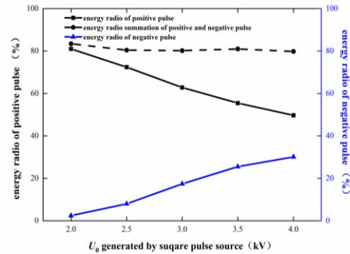
Fig. 11. The radio distribution of positive pulse energy and negative pulse energy to the whole pulse energy respectively.
