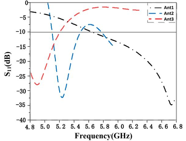
Fig. 3. Simulated  $|S_{11}|$  of Ant 1, Ant 2 and Ant 3.
