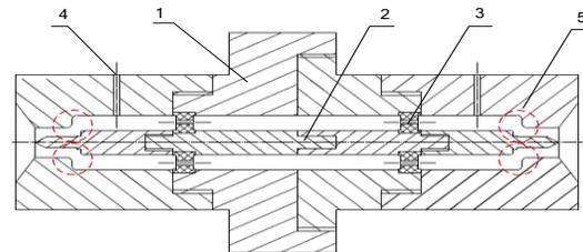
Fig. 1. Schematic diagram of the coaxial fixture.
