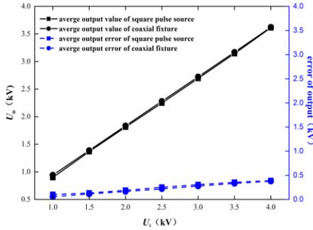
Fig. 8. Average output value and error of square pulse source and coaxial fixture respectively.
