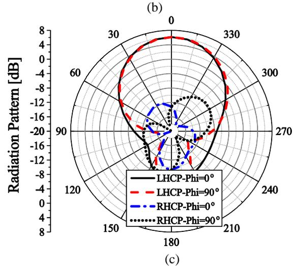
Fig. 4. (a) The simulated  $S_{11}$ , (b) AR and broadside gain, and (c) the radiation pattern at 5.3GHz of the proposed antenna.
