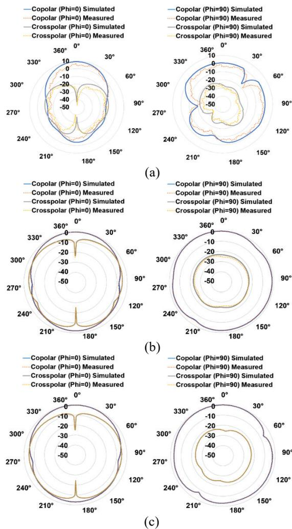
Fig. 6. Measured radiation patterns (E & H planes) of the proposed antennas at: (a) 28 GHz; (b) 24 GHz, and (c) 10 GHz.
