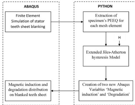
Fig. 7. Flowchart of the magneto-mechanical coupling process.
