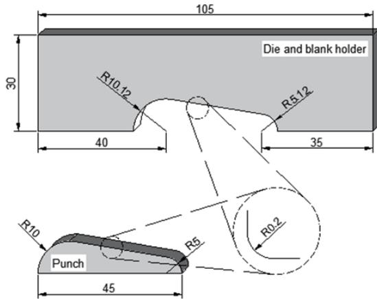
Fig. 3 Geometric description of the blanking tools.
