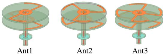
Fig. 2. Three improved prototypes of the proposed antenna.
