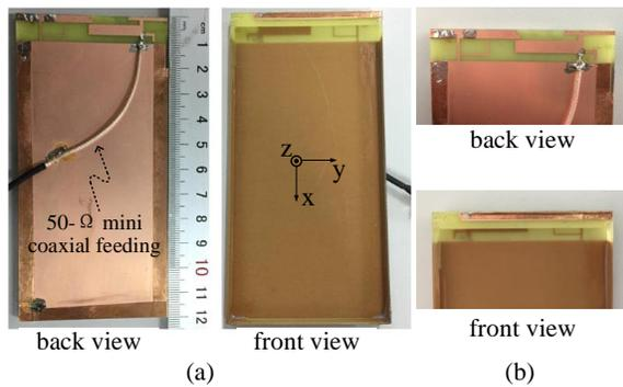
Fig. 8. Photographs of the fabricated antenna. (a) Overall view and (b) enlarged view.
