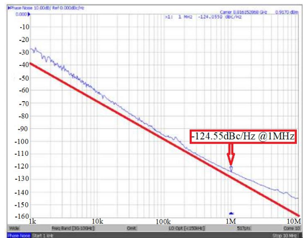
Fig. 6. Measured phase noise. V_{DD}=2\text{V} , V_{B1}=0\text{V} , V_B=2\text{V} . L_{\text{choke}}=4.7\text{nH} . A 1/f^3 guideline is used for reference.
