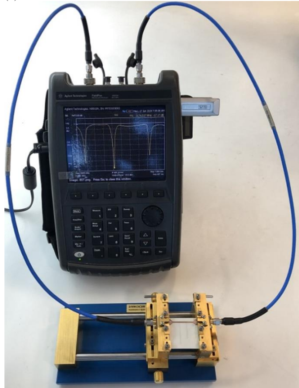
(b) Measurement of the transmission coefficient |S_{21}| using the VNA
