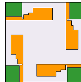
Fig. 3. Antenna 4 integrated by four antenna 3.
