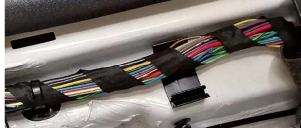
Fig. 1. Handmade cable bundles under car window.
