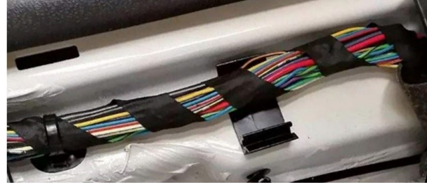
Fig. 1. Handmade cable bundles under car window.
