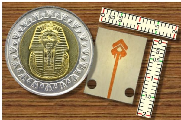
Fig. 2. Fabricated prototype of the proposed quad-band patch antenna with its size compared to a metal coin of standard size.
