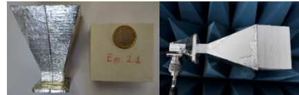
Fig. 4. 3D printed antenna design.
