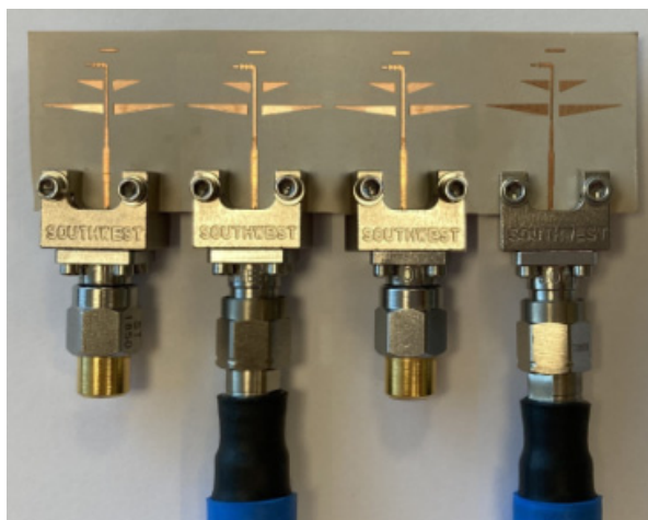
Fig. 21. Fabricated linear array composed of four elements of the proposed Yagi-Uda antenna.
