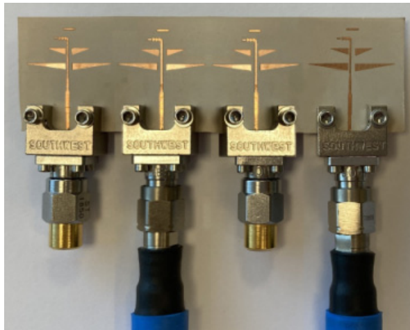
Fig. 21. Fabricated linear array composed of four elements of the proposed Yagi-Uda antenna.
