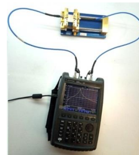
(b) The test fixture connected to the VNA
