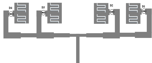
Fig. 4. The proposed array with PIN diodes located at QLR inputs.
