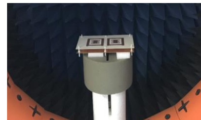
Fig. 11. Far-field measurement undertaken inside SATIMO.
