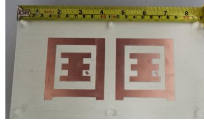
Fig. 9. Photograph of CP MIMO with closely packed ( D = 80 mm) Guo -shaped patch antennas.
