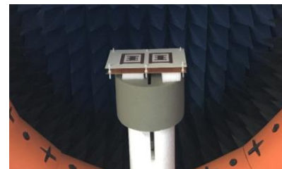
Fig. 11. Far-field measurement undertaken inside SATIMO.
