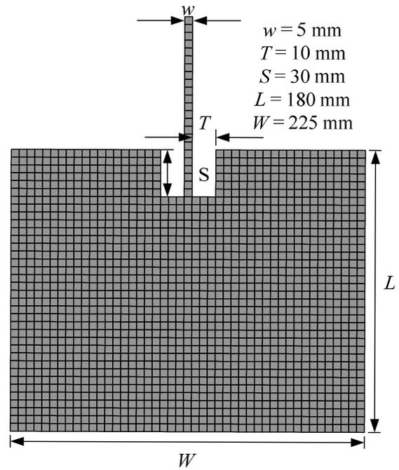
Fig. 5. Library structure of a planar patch.
