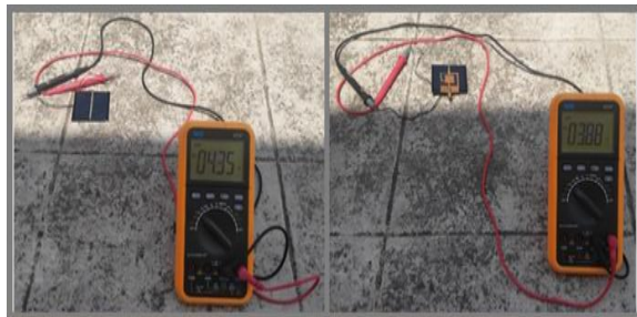
Fig. 10. Measurement of V OC and I SC of the solar cell with and without antenna integration.
