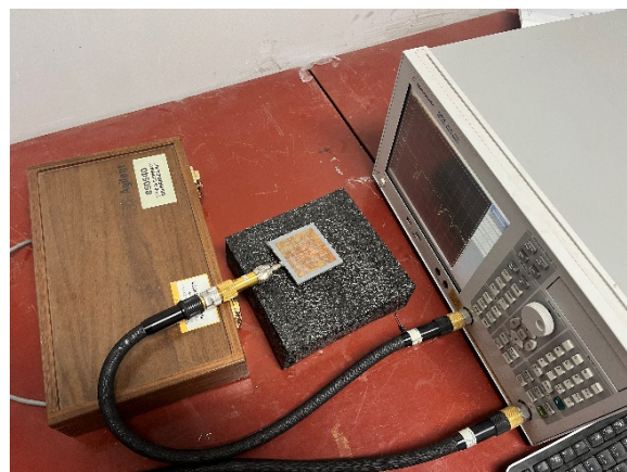
Fig. 11. The measurement of the proposed filtering antenna.
