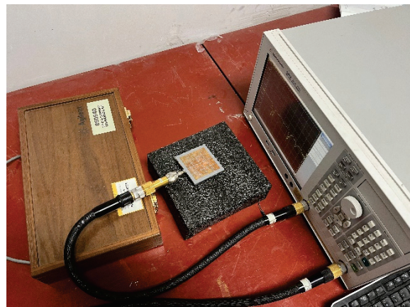
Fig. 11. The measurement of the proposed filtering antenna.
