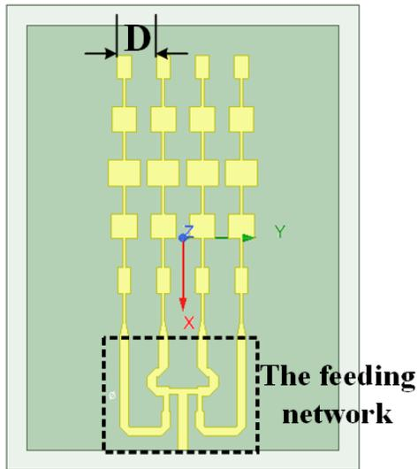
Fig. 2. The structure of the 5×4 planar array antenna.
