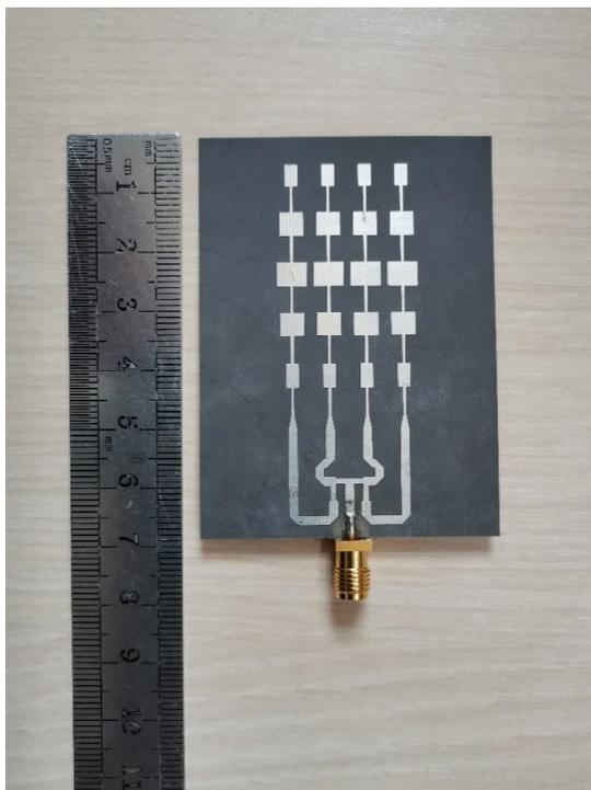
Fig. 3. The fabricated planar array antenna photograph.
