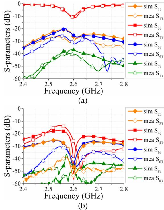
Fig. 9. Simulated and measured S-parameters of the  $1 \times 4$  full-duplex antenna array using the field-circuit combined method (decoupling network and ADS). (a)  $S_{13}$ ,  $S_{33}$ ,  $S_{53}$ , and  $S_{73}$ . (b)  $S_{23}$ ,  $S_{43}$ ,  $S_{63}$ , and  $S_{83}$ .
