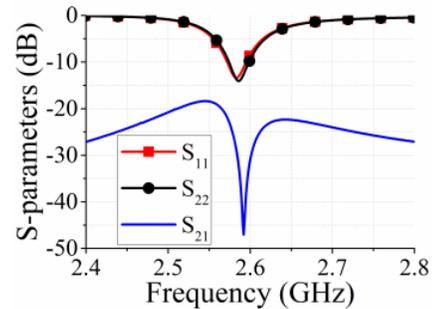
Fig. 2. Simulated S-parameters of the full-duplex antenna.
