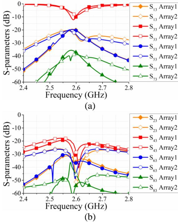
Fig. 5. Simulated S-parameters of the  $1 \times 4$  full-duplex antenna array with/without the decoupling network. (a)  $S_{13}$ ,  $S_{33}$ ,  $S_{53}$ , and  $S_{73}$ . (b)  $S_{23}$ ,  $S_{43}$ ,  $S_{63}$ , and  $S_{83}$ .
