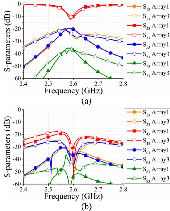
Fig. 6. Simulated S-parameters of the  $1 \times 4$  full-duplex antenna array with/without the decoupling network and ADS. (a)  $S_{13}$ ,  $S_{33}$ ,  $S_{53}$ , and  $S_{73}$ . (b)  $S_{23}$ ,  $S_{43}$ ,  $S_{63}$ , and  $S_{83}$ .
