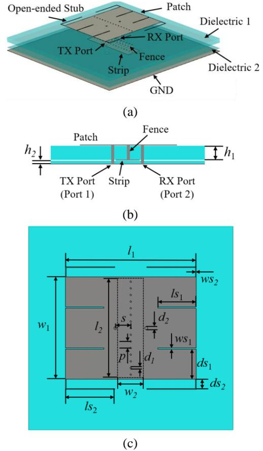
Fig. 1. Configuration of the full-duplex antenna. (a) Perspective view. (b) Side view. (c) Top view. The optimized parameters are:  $h_1 = 3$ ,  $h_2 = 0.165$ ,  $l_1 = 50$ ,  $l_2 = 40$ ,  $w_1 = 39$ ,  $w_2 = 10.4$ ,  $l_{s1} = 12.6$ ,  $l_{s2} = 19.2$ ,  $ws_1 = 0.5$ ,  $ws_2 = 0.3$ ,  $ds_1 = 11.25$ ,  $ds_2 = 4$ ,  $d_1 = 0.6$ ,  $d_2 = 1$ ,  $s = 6$ ,  $p = 2.6$  (all dimensions in mm).
