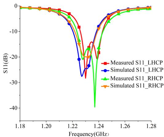
Fig. 11. The simulated and measured S11 of the L/RHCP microstrip antenna.
