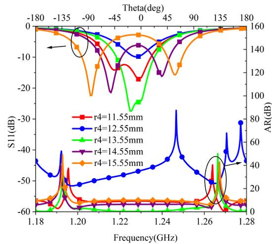
Fig. 8. S11 and AR with variation of  $r_4$ .
