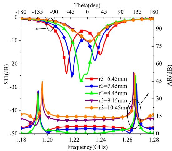
Fig. 7. S11 and AR with variation of  $r_3$ .
