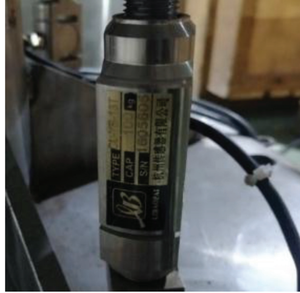
Fig. 2. CL-YB-13T/100kg force measuring sensor.
