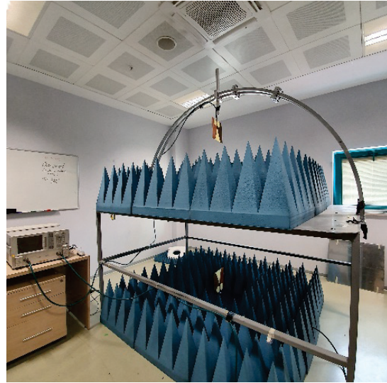
Fig. 8. The measurement room and measurement setup.
