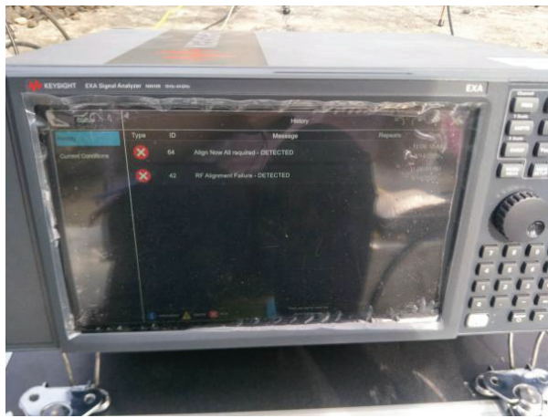
Fig. 14. Damaged spectrum analyzer.
