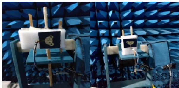
Fig. 7. Antenna measurement inside the chamber H -plane E -plane E -plane orientation (left) H -plane orientation (right).
