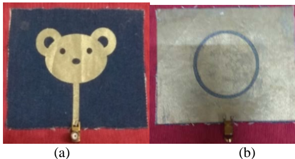
Fig. 4. Antenna topology. (a) Front view. (b) Back view.
