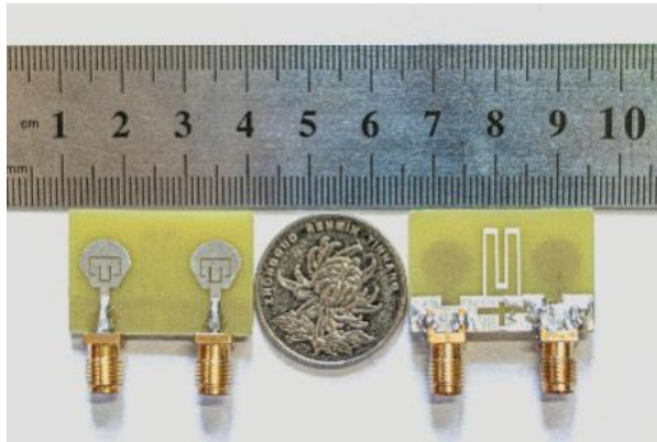
Fig. 9. Fabricated prototype of proposed two-port MIMO antenna.
