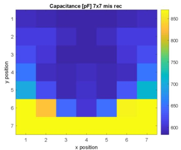
Fig. 7. Values of the tuning capacitors in the metasurface with  $7 \times 7$  elements.
