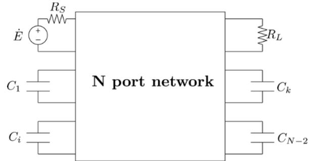
Fig. 2.  $N$ -port circuit representation of the proposed WPT system:  $N-2$  ports are dedicated to the capacitive loads of the metasurface unit cells, while the first two are relative to the transmitting and receiving coils.
