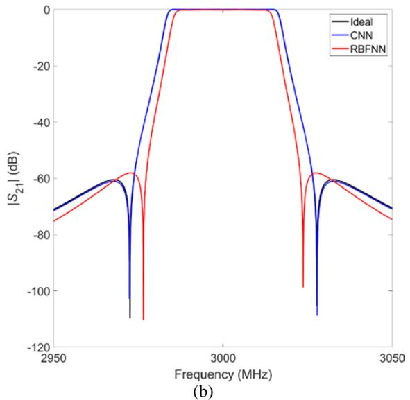
Fig. 4. The responses calculated by the coupling values in Table 3: (a) Return loss and (b) insertion loss.
