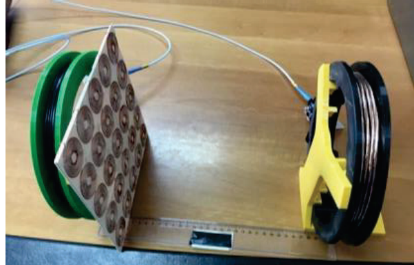
Fig. 3. Experimental setup. The metasurface is placed few millimeters above the driving coil.
