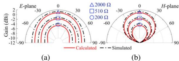
Fig. 6. Calculated and simulated gain patterns at 5.8 GHz of the infinite-ground model under different loaded resistance: (a) E-plane patterns and (b) H-plane patterns.
