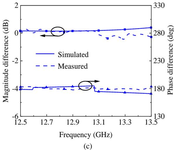
Fig. 6. Simulated and measured results of proposed four-way SIW FPD: (a)  $S$ -parameters, (b) magnitude difference and phase difference of in-phase case, and (c) magnitude difference and phase difference of out-of-phase case.
