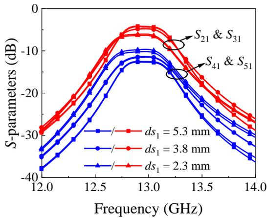
Fig. 5. The PDR changes under different parameters  $ds_1$ .
