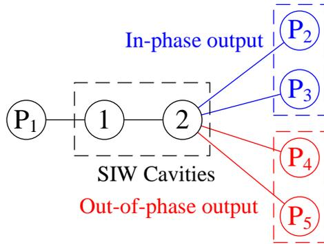
Fig. 2. Coupling diagram of proposed four-way SIW FPD.
