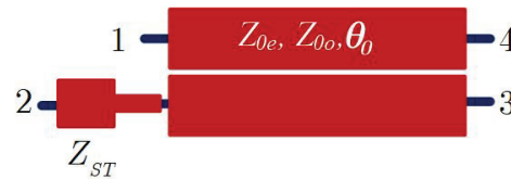
Fig. 4. The proposed coupled lines based SITL compensated coupled lines.
