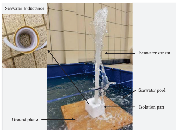
Fig. 8. The seawater antenna with isolation part.
