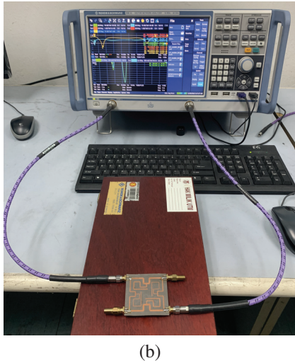
Fig. 8. The structure of the fabricated prototype for BLC-2 (a) with SMA connectors and (b) with VNA during S-parameter measurement.
