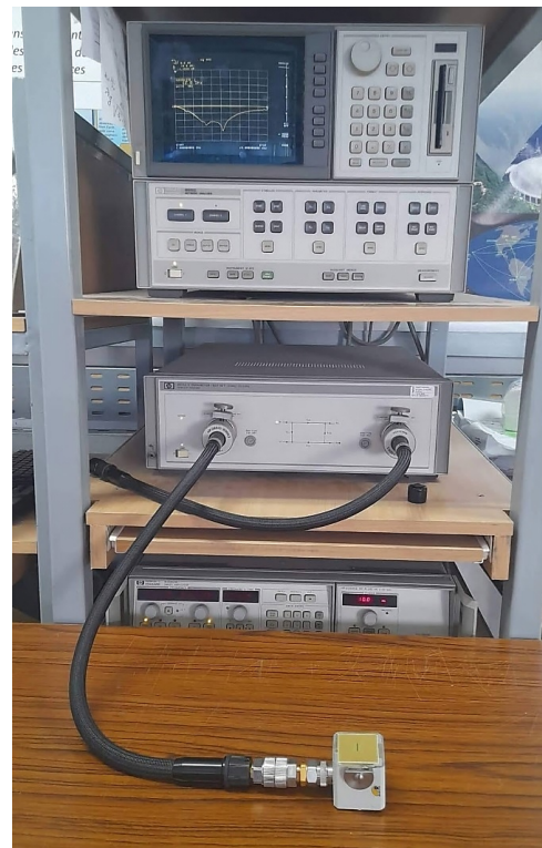
Fig. 12. Photograph of measurement set-up: Reflection coefficient measurement.
