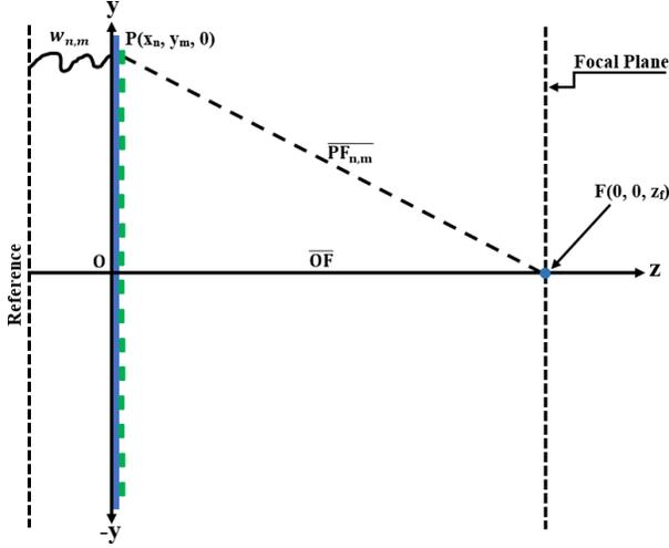
Fig. 2. The geometry of the focusing antenna array.
