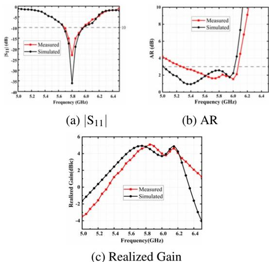
Fig. 9. Simulated and measured result for the proposed antenna. (a)  $|S_{11}|$ ; (b) AR; (c) Realized gain.
