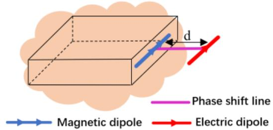
Fig. 2. Schematic diagram of the proposed antenna.
