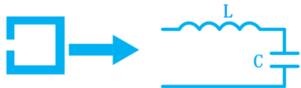
Fig. 4. Equivalent LC circuit of the SRR.
