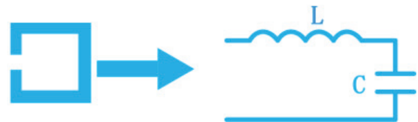
Fig. 4. Equivalent LC circuit of the SRR.
